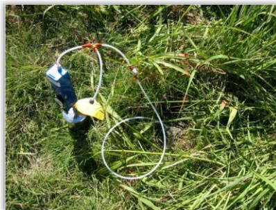
Temporary Soil Gas Probe
